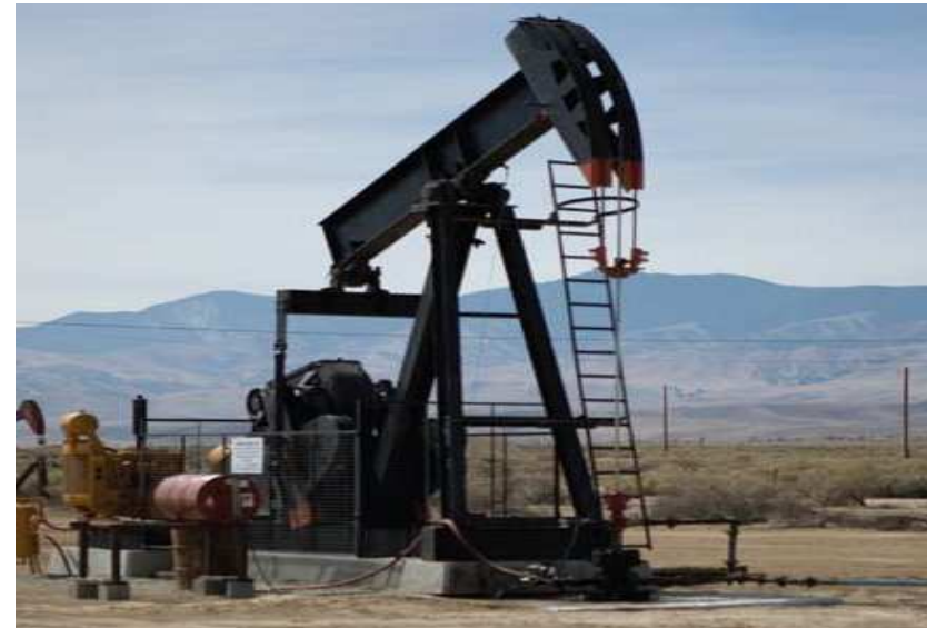
Beam pump on oil producer Maricopa - 6
